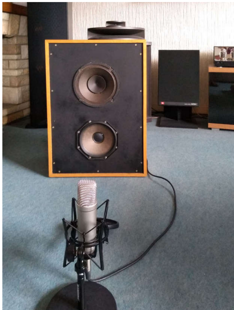
Photo: Measuring the frequency response of an old Philips 9710M.
